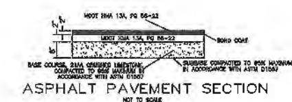
ASPHALT PAVEMENT SECTION NOT TO SCALE
